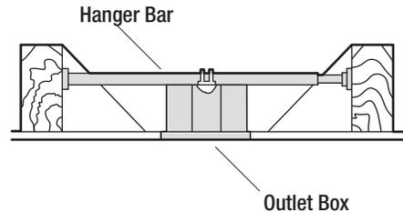
To hang your fan where there is an existing fixture but no ceiling joist, you may need an installation hanger bar (not included) as shown above.
