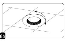
Spin the downlight a bit, to ensure the trim is flush against the ceiling.
