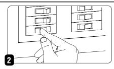
Before starting the installation process, TURN OFF POWER at the source of the housing(s) that you are installing fixture(s).
