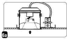
Push Downlight fixture into recessed housing.
