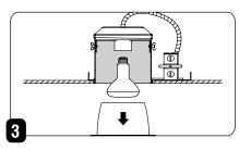
Remove existing trim and bulb, revealing the existing socket.
