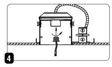
Thread the socket adapter into the socket.
