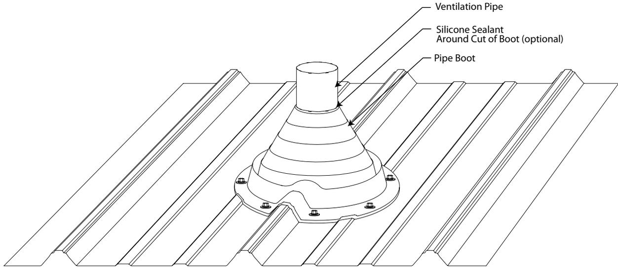
1-1/2" Screws Spaced 1" Around Base of Pipe Boot
