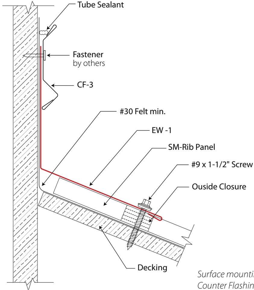
*Surface mounting requires use of Counter Flashing (CF-3)*
