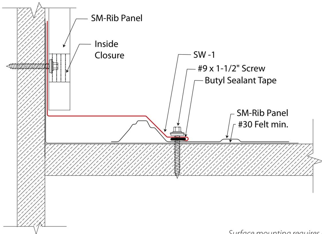
*Surface mounting requires use of Counter Flashing (CF-3)*
