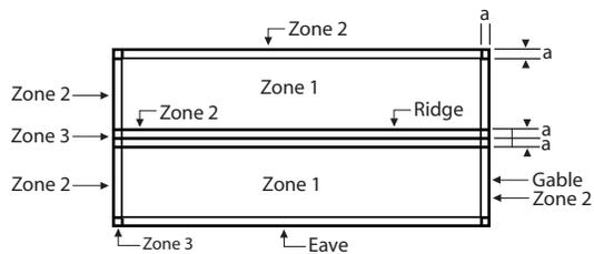
Note: Dimension (a) is defined as 10% of the minimum width of the building or 40% of the mean height of the roof, whichever is smaller, however, (a) cannot be less than either 4% of the minimum width of the building or 3 feet.
