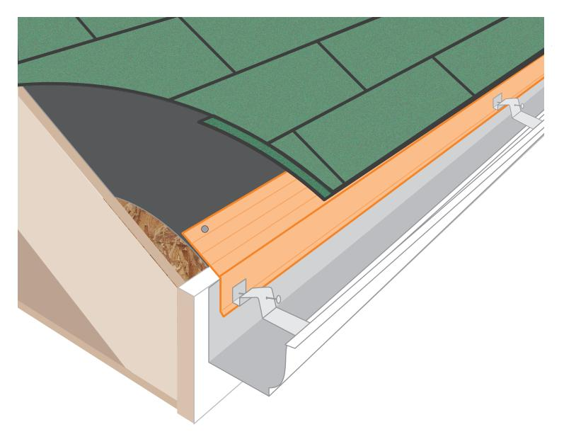
The 3 inch top section is installed under the starter shingle course and above the underlayment. The gutter apron flashing is secured with roofing nails every 16-24 inches. Overlap joints a minimum of 2 inches.
