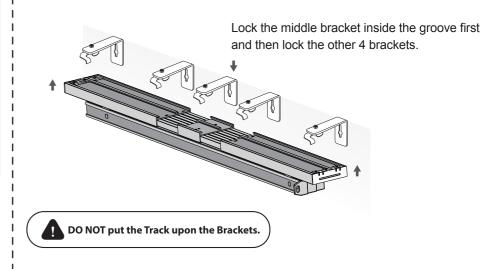
**Step 5** Make sure the mounting brackets are tightened inside the groove.
