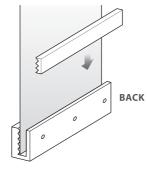
**e** Use Allen wrench to screw set screws into the bottom rails.
