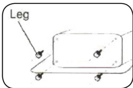
If the floor is uneven, adjust the legs, do not insert pieces of wood, or any other objects under the legs. Adjust the height level of the legs accordingly.
