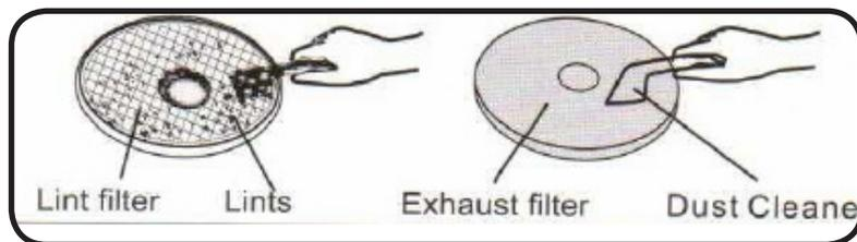
Separate each of the above parts and clean the individual pieces using a soft brush or vacuum cleaner. **DO NOT** damage the filters.
