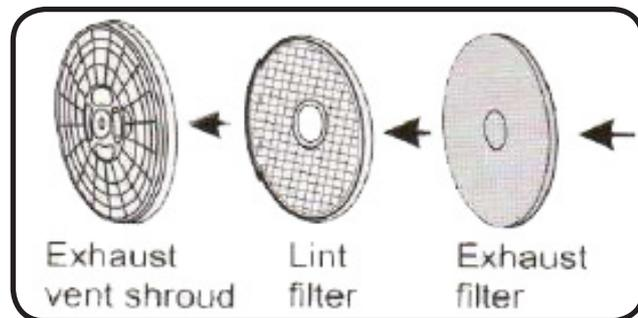
Separate each of the above parts and clean the individual pieces using a soft brush or vacuum cleaner. **DO NOT** damage the filters.
