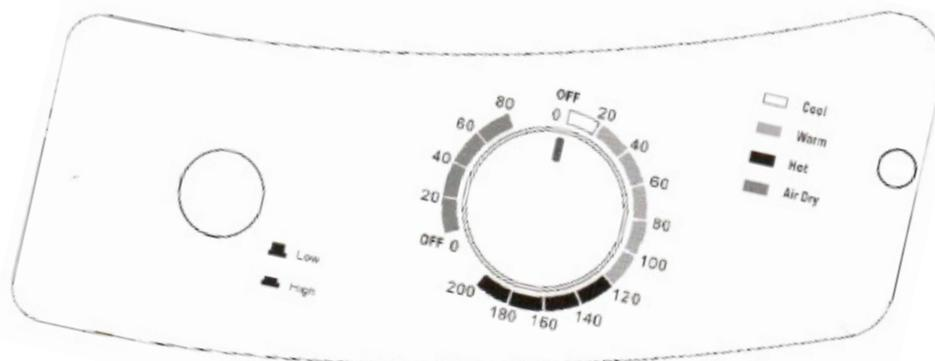
**Air Dry:** This function runs with cool air, primarily to air items that require freshening i.e.: clothes that have been stored for a long period of time.
