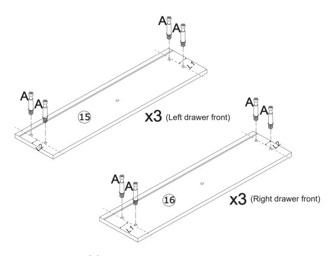
L1: Longer Hole-To-Edge Distance L2: Shorter Hole-To-Edge Distance
