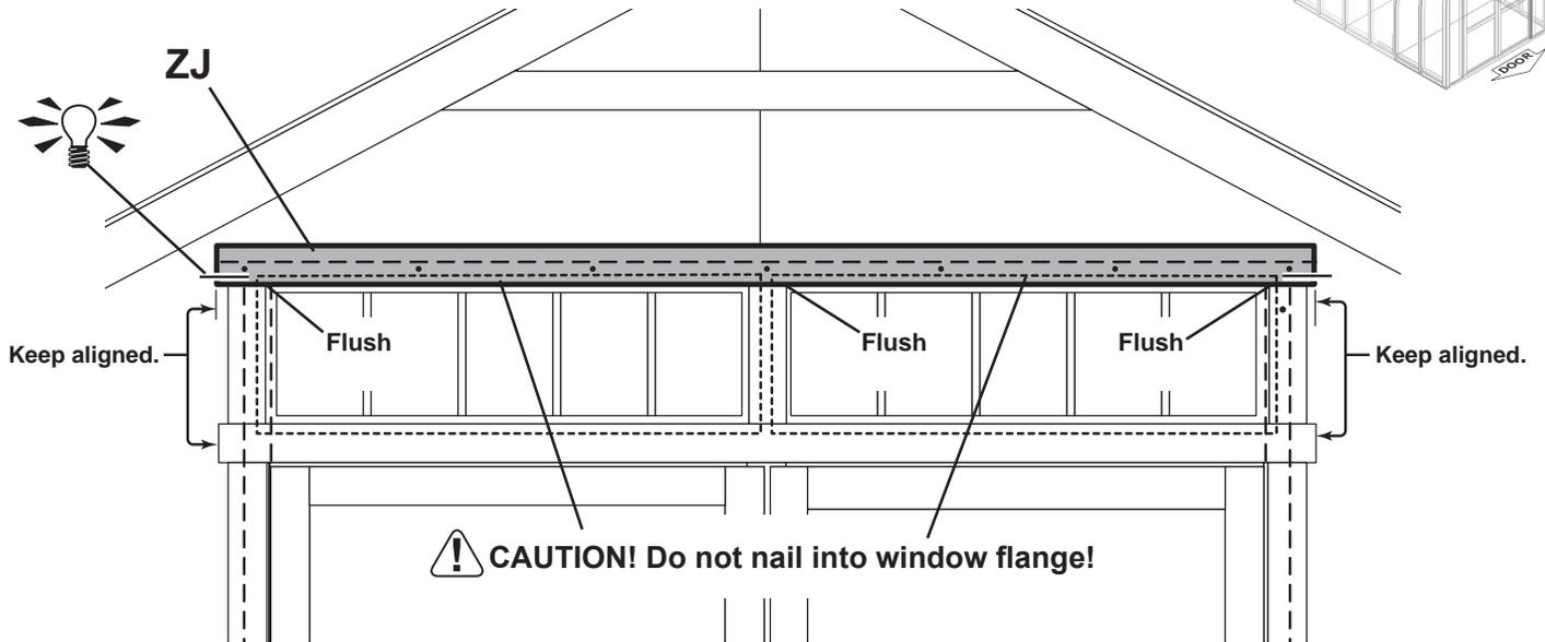
**7** From inside, install 3/4" screws into **ZJ** and outer two **EY**.
