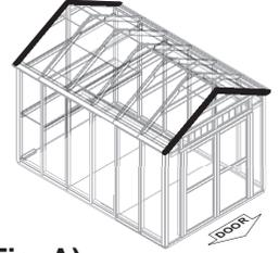
**NOTE:** Upper gable panels may be slightly offset from lower panels. If this occurs, mark a line on upper panel to match lower wall panel (Fig. B).
