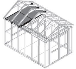
**1** Place loft panels onto the three loft supports centered from side-to-side and flush with the back wall panel. Fit panels into gap.
