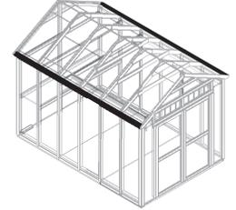
**2** Secure ends of **TP** and **AN** with (2) 3" screws through gable trim (**Fig. A**).
