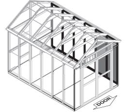
**3** Place the 48 x 84" panel onto wall frame with primed side up as shown.
