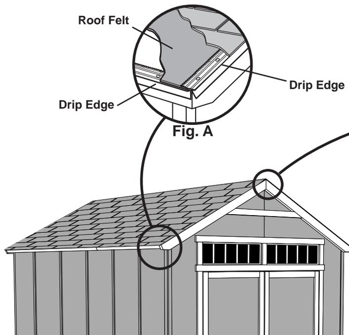
Snip bottom side of drip edge and bend over to other side of roof.
