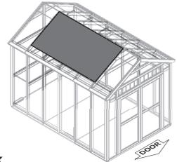
You must square the roof by attaching one panel first. You will use the panels' long edge as a lever to bring your roof into square. Commonly known as "racking".
