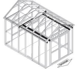
**3** Place **PT** against loft support (**Fig. A**) and secure flush using two 3" screws.
