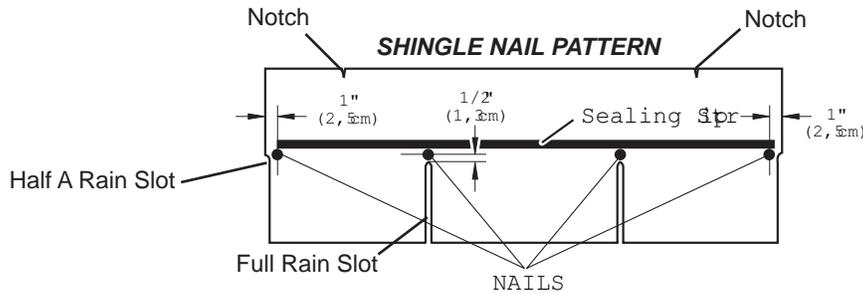
**!** NEVER DRIVE FASTENERS INTO OR ABOVE SEALING STRIPS.
