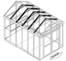
**2** First, secure ends of rafters with one 2" screw at each end (Fig. A). Secure ends of rafters with two 3" screw at each end (Fig. B, Fig. C).
