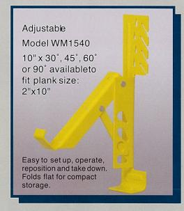
Can be easily installed and removed without damaging shingles. The capacity of scaffolding support models is one worker per 8 foot staging plus 40lbs., with a maximum of 8 feet between brackets.
