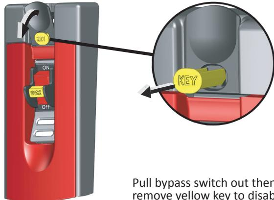
Pull bypass switch out then remove yellow key to disable bypass. Insert yellow key to re-enable.
