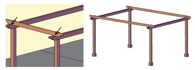
**Step 4.** Attach main knee brace to post & dual support beam with two bolts, washers & nuts. (Match numbers). Tap the bolt all the way into the wood to set it, then add a washer and nut and lightly tighten. Repeat this step with the other main knee braces.
