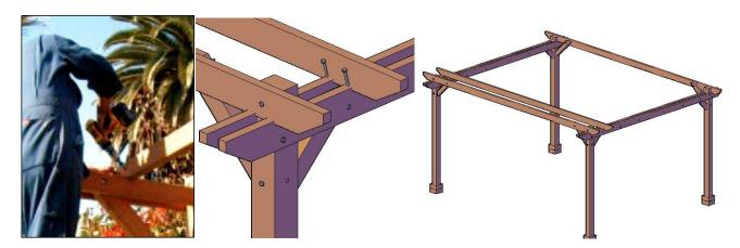
**Step 6.** Attach roof slats to rafters with deck screws (2 ½ "). The roof slats are all marked with ink as well as a predrilled hole to use wood screws. The rafter tops are marked in ink with 2 lines. Place one roof slat into the lines on one end and begin to attach. *And repeat the process in all roof slats*.
