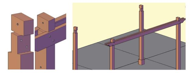
**Step 3.** Attach corner rafter to posts with one bolt per post (7 " x 5/16") washers & nuts. (Match numbers). Tap the bolt all the way into the wood to set it, then add a washer and nut and lightly tighten.
