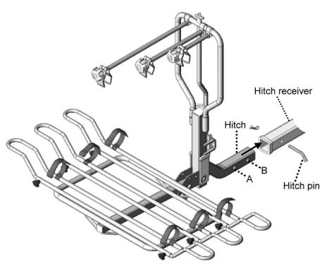
**Clamp Arms:** Adjust each clamp to fit your bike frame and tighten the knob securely.
