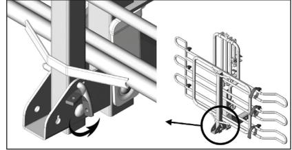
**Step 4.** Insert the assembled sections (A and C) into the hitch mount (F). Attach using the M12x76 carriage bolt (B2) and nut (N2).
