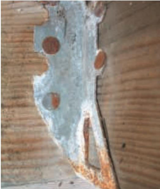
Galvanized joist hanger attached to ACQ wood, 7 months; wet conditions.
