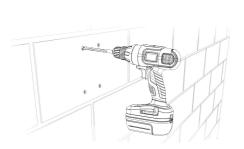
Use the template provided in this instruction manual to mark hole location on a sturdy wall
