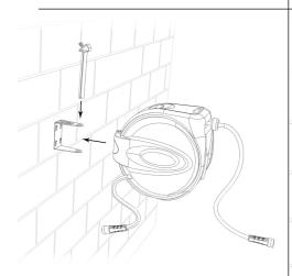
Align Power Reel mounting hole with holes in bracket. Slide Pin through all holes to secure. Unit should rotate freely
