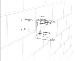
Insert the anchors provided into the 4 holes. They should be flush with the wall. Use the provided screws to attach bracket
