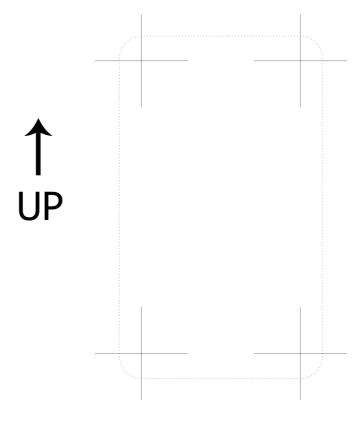
Mark the wall where you are mounting your Retractable Power Hose Reel at the center of the four crosshairs.
