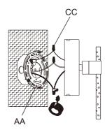
4. Place fixture body (A) onto the mounting plate (AA), securing with previously removed flat head screws (DD).
