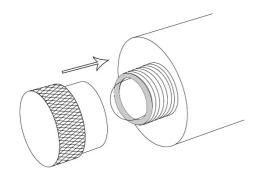
**Step6**–Install O-ring onto the closed end of the quartz tube.
