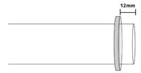
**Step 5**—Insert the quartz tube into the Filter chamber.
