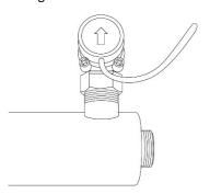
**Step 13**—Connect flow switch cable with control switch, close the switch cover.
