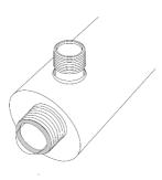
**Step8** –Hand-screw open end nut on the filter chamber (open end of quartz tube). To protect the O-ring, do not over tighten.
