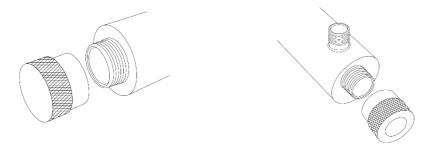
**Step4**–Install O-ring onto the open end of Quartz Tube (12mm from the edge).
