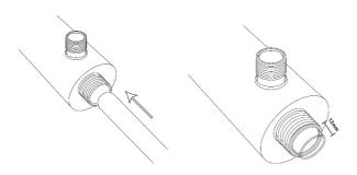
**Step7**–Hand-screw closed end nut on the filter chamber(closed end of quartz tube). To protect the O-ring, do not over tighten.
