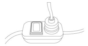
**Step 14**—Push control switch to button "AUTO", the UV lamp will starts working automatically when there only water flowing. Push control switch to button "MOVE", the UV lamp keep working continuedly. Push control switch button "STOP" to turn off the UV lamp. Mode AUTO is highly recommended to protect the UV lamp.
