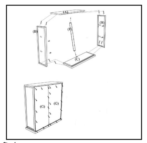
**Step 1**Combine the Top (A), Side Board (B), and Post(F) with the Base (C), use Allen Key to tighten all the bolts.
