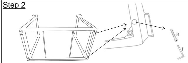
Attach the second Side Panel with Handrail(C) to Bottom Shelf(B) using Bolt(H) with Allen Key(I).
