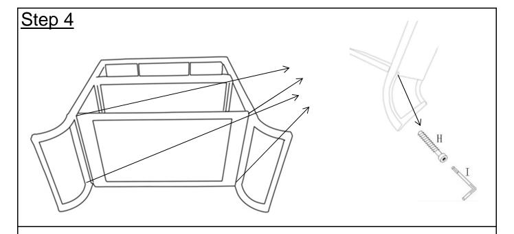
Attach Top Shelf(A) to between Side Panels with Handrail(C) using Bolt(H) with Allen Key(I).
