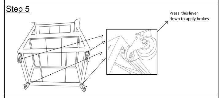
Turn-in Wheels(G&J) by hand, into the four Mounting Positions.
