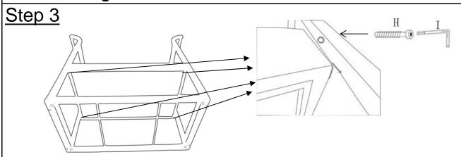
Attach Middle Tray(D) between Side Panels with Handrail(C) using Bolt(H) with Allen Key(I).
