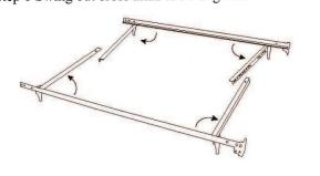
Step 2 Place rivets of the cross arms into appropriate key holes then slide to lock as shown in Figure 1.
