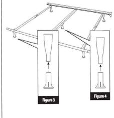
Step 5 Place support legs under holes that align on center of cross arms .Screw in as shown in Figure 5. Use bolts NO1.
