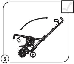
5 Set the unit upright. Loosen the knobs. Swing the handlebar up into the operating position.
