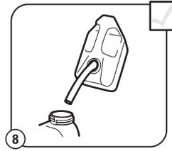
8 Position the unit with the fuel cap facing up. Slowly remove the fuel cap. Fill the fuel tank. Reinstall the fuel cap. Move the unit at least 30 ft. (9.1 m) from the fuel container and the fueling site before starting the engine.
