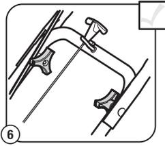
6 Tighten the knobs securely. Readjust the cables so they are smooth and tight against the handlebar.
