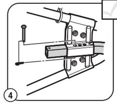
4 Insert the clevis pin through the wheel bracket and assembly and lock it in place with the cotter pin.
