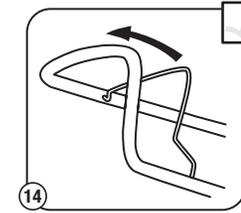
14 Squeeze the throttle control as needed for operation.
