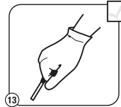
13 Pull the starter rope with a controlled and steady motion until the unit starts.
