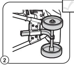
2 Set the unit on its side. Insert the wheel assembly into the wheel bracket.
