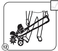
12 Stand in the starting position. Hold the handlebar firmly with one hand. Hold the starter rope with the other hand. Use one foot to hold the wheels in place. Tilt the unit back slightly to bring the tines off the ground.
