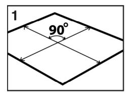
1. Calculate the center of the space by measuring the length and width; divide the dimensions in two. Mark the center of the space to identify the approximate starting point for the installation.
