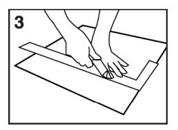
3. Upon reaching the edges, you may need to cut the tiles to fit within the desired space. To cut the tile, simply use a heavy duty utility knife. To fit tiles around irregular shapes (i.e. pipe), make a pattern from cardboard or heavy paper. Trace the pattern onto the tile and then cut with the utility knife.
