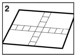
2. Begin to lay the tiles from the center point of the space in both directions towards the edges. Fill in each of the four quadrants that you've created.
