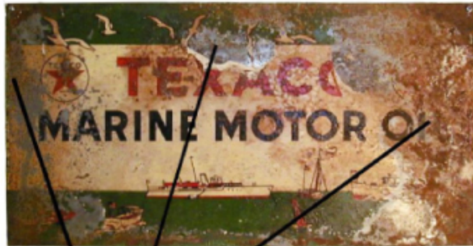
Rust behind paint removed
