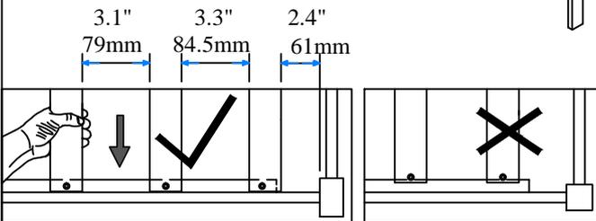
Note: Do not lock the screws of the bed slats to the outermost edge of the bed slats, you need to leave a certain space at the edges, otherwise it will cause the board to break. Do not lock the bed slats on the edge of the wood, please hold firmly before screwing, hold it in place with one hand, then lock the screw.
