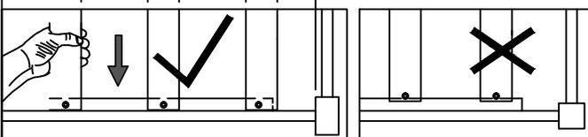
Note: Do not lock the screws of the bed slats to the outermost edge of the bed slats, you need to leave a certain space at the edges, otherwise it will cause the board to break. Do not lock the bed slats on the edge of the wood, please hold firmly before screwing, hold it in place with one hand, then lock the screw.
