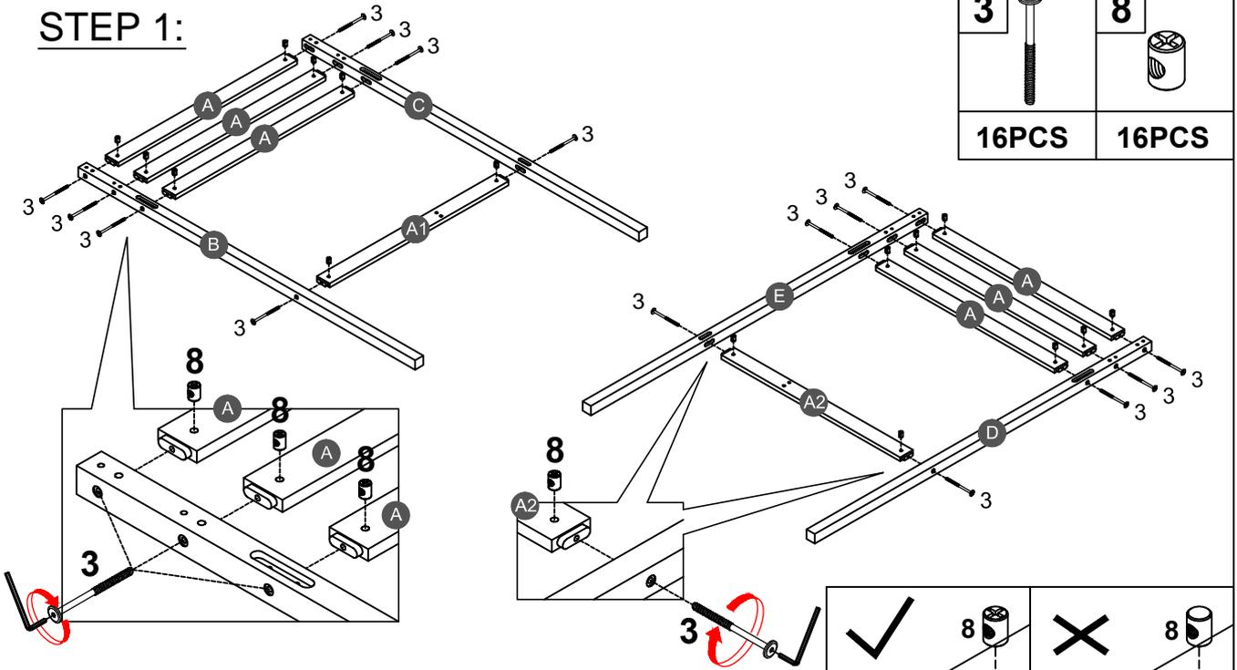
Note: Part 8 will face up with the "x" mark on it, otherwise it cannot be tightened
