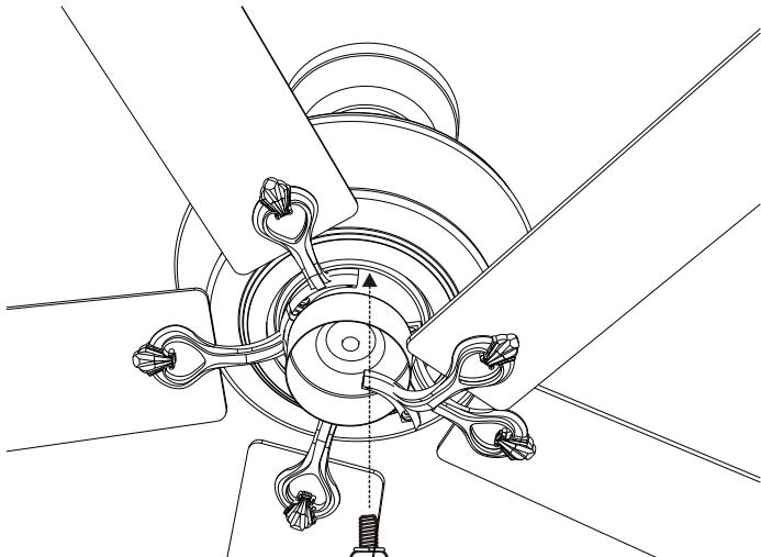
**NOTE:** Your fan features revolutionary advancements for quick and easy blade installation. Including an alignment post and captive blade arm screws.
