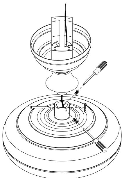
1. Thread the suspender through the suspended clock and coupling cover .
