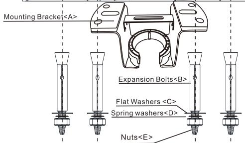
For concrete ceiling, use the percussion bit with diameter 8mm to drill holes according to the length of expansion screws. Then use the attached expansion screws to fix the hanging bracket onto the ceiling (selection is made according to actual requirements of the customers).
