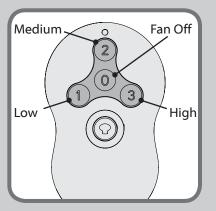
The Fan Off button only turns the fan off. To turn the fan on, press one of the fan speed buttons.
