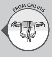
**CONNECT WIRES FROM RECEIVER TO WIRES FROM OUTLET BOX** - Using an orange wire connector connect the black wire (ungrounded) from the ceiling to the black wire from the receiver (marked "live in"). Connect the white wire (grounded) from the ceiling to the white wire from the receiver (marked "neutral in").
