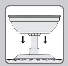
Remove the canopy. If uncertain how to remove it, reference the fan's owner's manual. With wiring exposed, it may be helpful to note existing wire connections or take a digital photo for reference. Remove the wire connectors that connect the wires from the outlet box to the fan, leaving the grounding wires connected.
