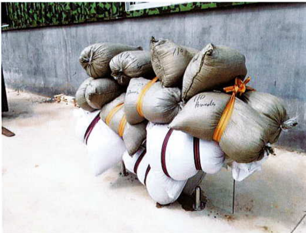
Photo 1: Panel loaded vertically with 2,520 pounds.
