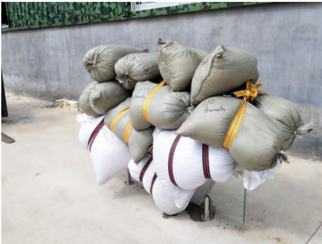
Photo 1: Panel loaded vertically with 2,520 pounds.
