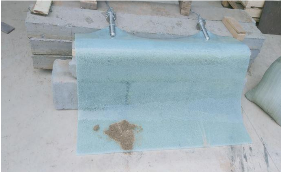
Photo 3: Panel after failure, showing all glass intact within laminate structure.
