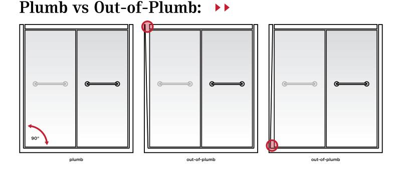
Most Delta Shower Doors are designed to accomodate out-of-plumb conditions up to 3/8". If your shower environment is out-of-plumb, simply adjust the placement of the roller to lower or raise the glass.
