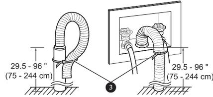
**Using a Laundry Tub to Drain**
