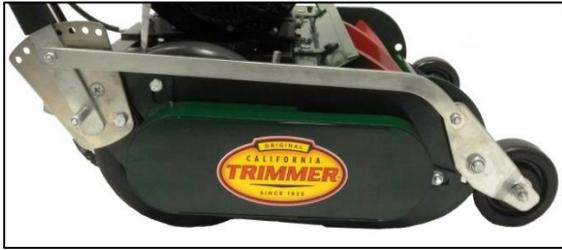
The front caster wheel axle comes standard in the middle position. It can be removed and placed in the bottom position to achieve additional settings for higher cutting heights. **NOTE: the top position would be used only for aftermarket caster wheels or front rollers that prevent access to the lower cutting heights in the middle position.**
