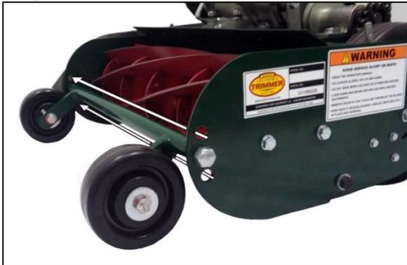
The height is changed by moving the adjustment handle into the positions of the bracket.
