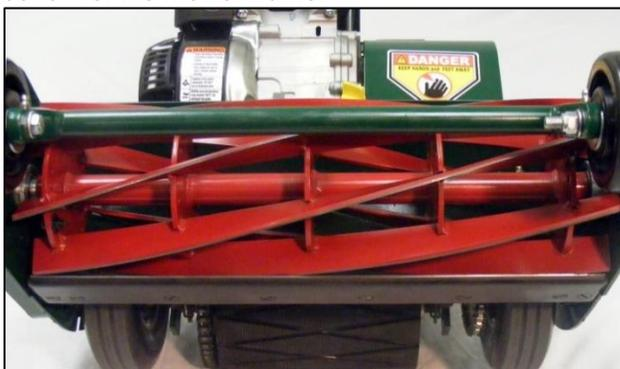
This function of the mower is pre-set at the factory, but based on the type of grass and other factors, further adjustment may be necessary. As the blade reel and bed knife wear, additional adjustment will be required.
