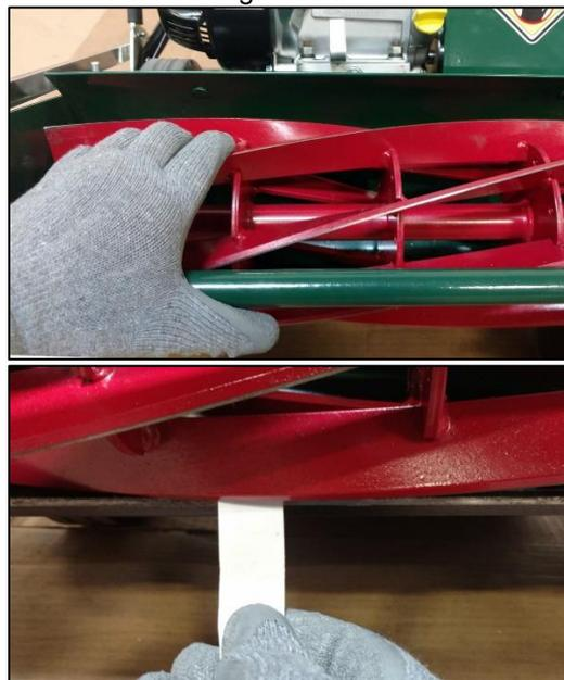
**NOTE: Excessive contact will cause overheating and damage to the parts.** Insufficient contact will not allow for the grass to be cut. Any excessive noise means that the adjustment is too tight. It is not recommended that the reel be engaged for extended periods of time when not cutting grass as the moisture provides a level of lubrication to the cutting surfaces while in use.
