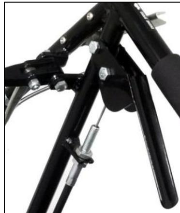
When disengaged, the belt tension is loose and it is in contact with the belt guide and belt guard to help prevent it from turning. If needed, the belt guide can be rotated to have more contact with the belt.
