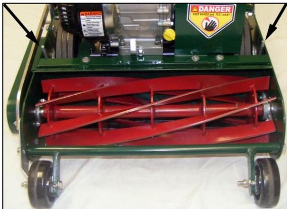
The adjusters raise and lower each side of the bed knife in relation to the reel, increasing or decreasing the clearance and should be moved as evenly as possible.
