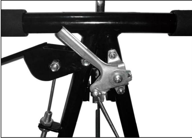
5. Secure the throttle wire using the holder clips on the handle. **Note: Use 1 or 2 clips depending on the routing.**
