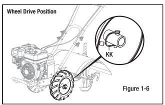
FOR FREEWHEEL MODE: Slide the wheel inward and insert the wheel drive locking pin (KK) only through the hole in the axle shaft. Secure wheel locking pin (KK) by pushing in as far as it will go then wrapping the ring around the wheel shaft as shown. Repeat for the other wheel and then remove the support from beneath the transmission.
