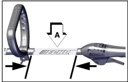
1. Position Support Handle (A) in comfortable operating position and tighten wing nut (B). The cutting attachment should be 5 cm to 7.5 cm (2 in. to 3 in.) above the ground and as level as possible.
