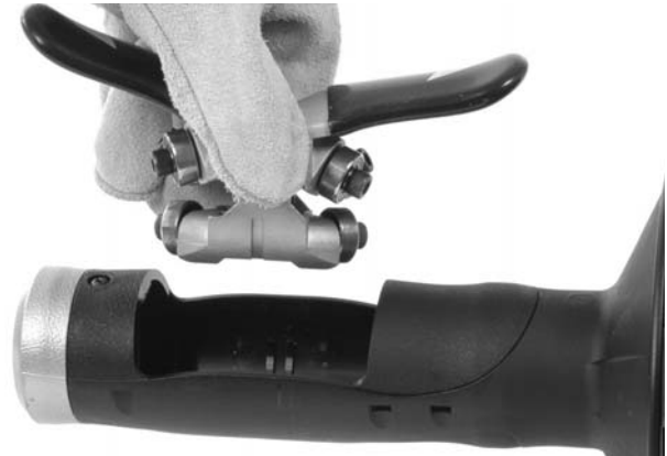
Figure 12B – Removing AUTOFEED Mechanism From Housing
