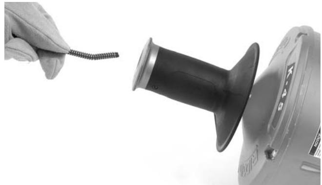
Figure 17 – Loading Cable Without Changing Inner Drum
