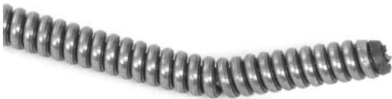
Figure 15 – Bend At Cable End
