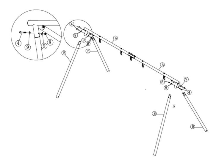
Insert the rest 4 Support Legs(#B) into sockets as shown, and attach the Cross Bar(#C). Align the hole and secure with M8\*50mm Bolt(#4), Flat Washer(#5), Arc Washer(#9) and M8 Nylon Nut(#8).
