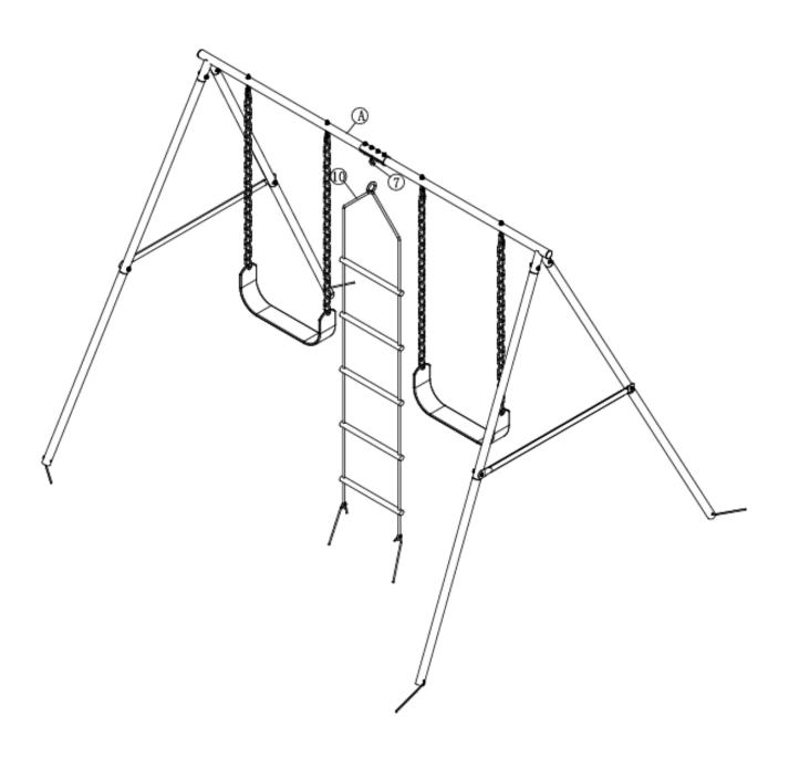
Now you have finished assembling your swing set. Go back and tighten all bolts and nuts securely before using the playset.
