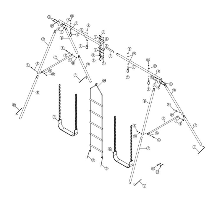
Connect 2 Top Bars(#A) together with Connecting Tube(#1), and then wrap the joint with Metal Bracket(#E) as shown.
