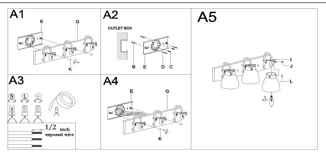
Step A1: Unscrew the knob nuts (K) from back plate(G) then gently remove mounting plate (E).
