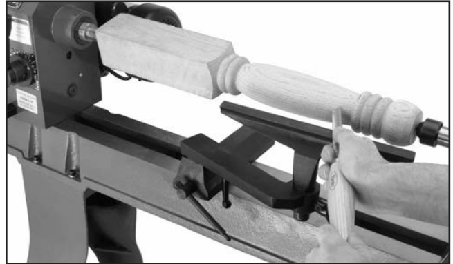
Figure 34. Typical spindle turning operation.
