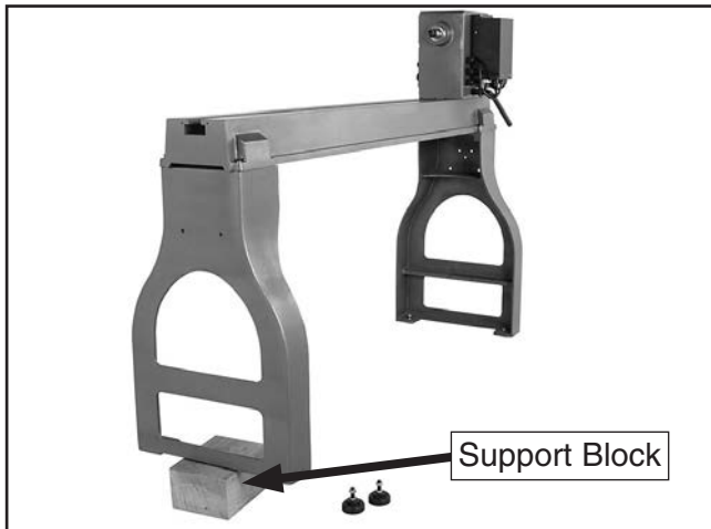
Figure 12. Legs supported for feet installation.
