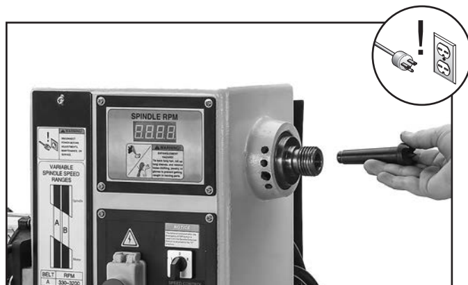
Figure 21. Installing center into the headstock spindle.
