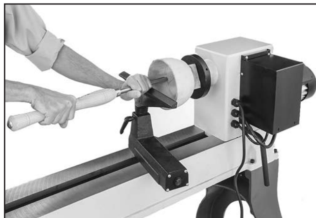
Figure 38. Typical faceplate turning operation.
