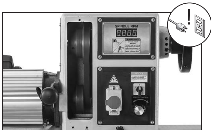
Figure 28. Belt access panel removed.
