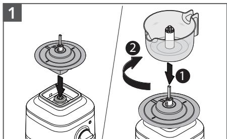
Place the Gear Assembly on base. Place the Juice Container on Gear Assembly and twist clockwise to lock in place.
