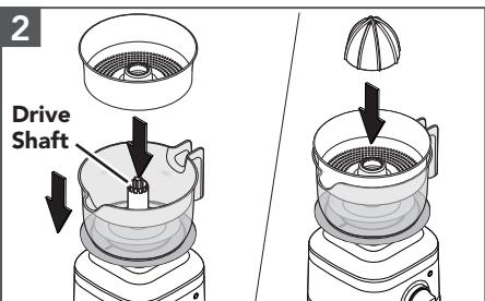
Place the Pulp Basket and then the Reamer into the Juice Container by aligning them with the Drive Shaft.
