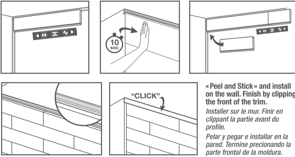
**«Peel and Stick» and install on the wall. Finish by clipping the front of the trim.**
