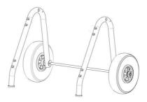
4. Use the screw (item 10), washer (item 9), and nut (item 8) to assemble the handle to the foot stand as shown below. Tighten the nuts.
