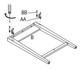
$\Box$  c) Join frame (B) to the assembled body with dowel (AA).
