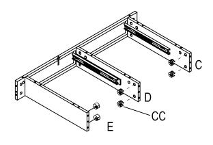
□ d) Tighten bolt (BB) with lock (CC) in the pre-drilled holes.
