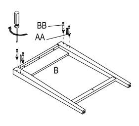
c) Join frame (B) and bar (H) to the assembled body with dowel (AA).
