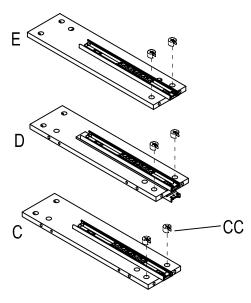
□ d) Tighten bolt (BB) with lock (CC) in the pre-drilled holes.
