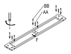
□ c) Join partitions (C), (D) and (E) to the panel (F) with dowel (AA).
