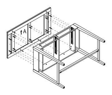
b) Insert lock (CC) into panels (G) and (F), and partitions (C), (D) and (E).
