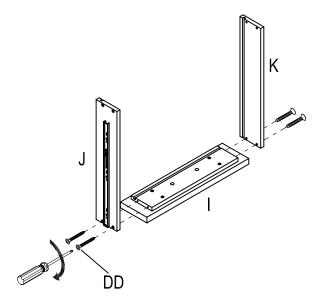
c) Tighten panel (L) to the assembled body with screw (DD).
