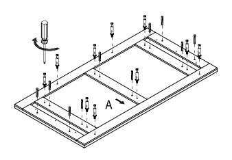
c) Join panel (A) to the assembled body with dowel (AA).
