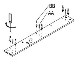
□ c) Join panel (G) to the assembled body with dowel (AA).
