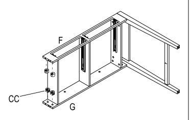
d) Tighten bolt (BB) with lock (CC) in the pre-drilled holes.
