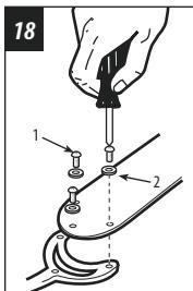
Attach blade brackets to blades using the blade bracket screws (1) and fabric washers (2).
