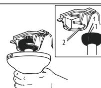
Carefully lift fan assembly onto mounting bracket. Rotate fan until notch on downrod ball (1) engages the ridge on the mounting bracket (2). This will allow for hands free wiring.
