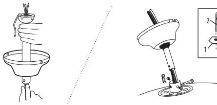
Feed motor lead wires through downrod/canopy assembly and insert downrod into downrod yoke. Make sure to align hole in downrod with the hole in downrod yoke. Install yoke cross pin (1) through yoke and downrod. Insert clamp pin (2) into cross pin until it snaps into place. Tighten set screws (3) in yoke.
