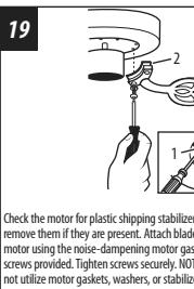
Check the motor for plastic shipping stabilizer tabs (1), and remove them if they are present. Attach blade assembly to motor using the noise-dampening motor gaskets (2) and motor screws provided. Tighten screws securely. NOTE: Some models do not utilize motor gaskets, washers, or stabilizer tabs.
