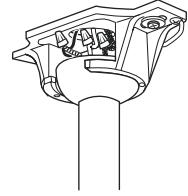
With bracket holding fan assembly, make electrical connections using the following step for wiring instructions.
