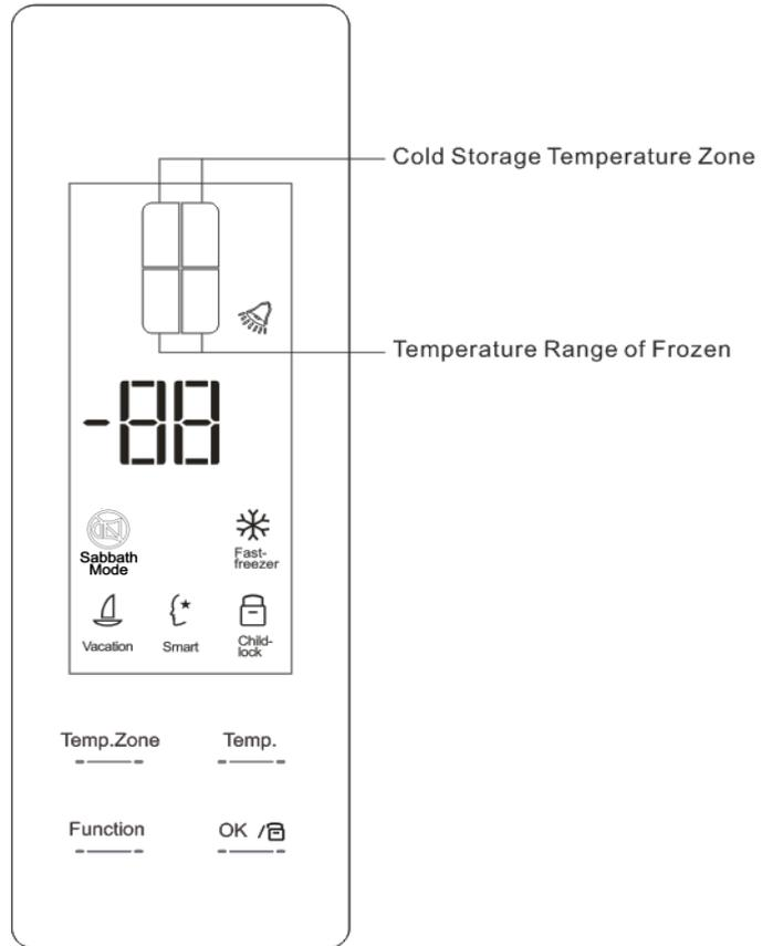
In fast-freezer state, press the "Function" key to "Fast-freezer" icon flashing, press the "OK" key, exit fast-freezer function; In fast-freezer state, into the "smart" refrigerator, automatic exit fast-freezer function.
