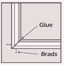
Must moldings are installed with a 90 degree angle joint. Cut 2 pieces of molding with a 45 degree angle each piece and together they make 90-degree angle. Use WPB Cement to glue the ends of the boards. On both sides place fasteners 2" from the end.
