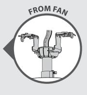
Connect wires from the receiver and fan to wires from the ceiling as shown. Using the wire connectors, connect the black wire (ungrounded) from the ceiling to the black wire from the receiver. Connect the white wire (grounded) from the ceiling to both the white wire from the receiver and the white wire from the fan. If you're uncertain about wire colors or connections, please contact a qualified electrician.
