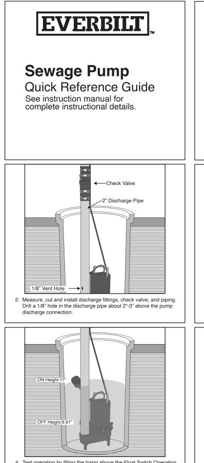
Test operation by filling the basin above the Float Switch Operation ON Height to make the pump start pumping out. When the water reaches below the Float Switch Operation OFF Height, ensure it stops pumping.
