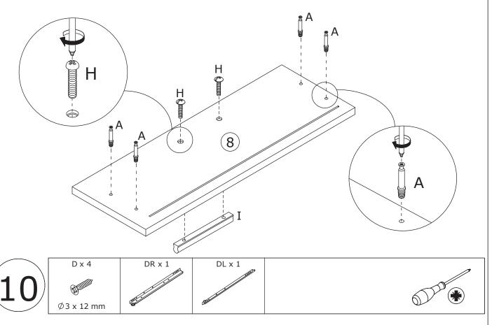
Fix runner(DL) and (DR) respectively to No.9 and No.10 plate using screw(D) as shown.
