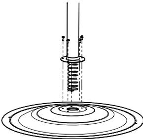
4. Place the fan head on top of the standing pole and secure in place using the long bolt and nut.
