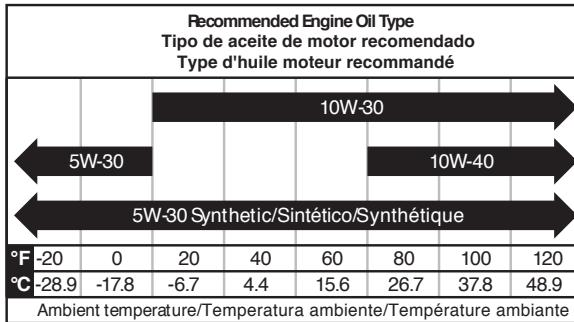
Only use 4-stroke/cycle engine oil. **NEVER USE 2-STROKE/CYCLE OIL.** Synthetic oil is an acceptable substitute for conventional oil.
