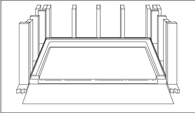
8. Apply a bead of 100% silicone sealant to seal the joint between the shower floor and shower floor ramp.
