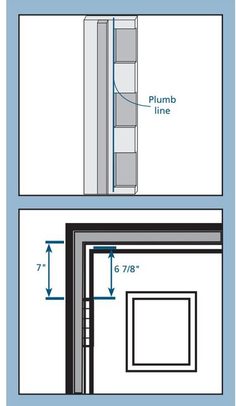
3. If installing new jambs, measure down from the underside of the top of the jamb (not the stop) 7" to position the top of the top hinge. Measure up from the top of the threshold 10" to position the bottom of the bottom hinge. Place the middle hinge halfway in between.
