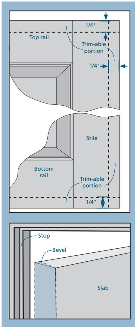
**TEST SLAB FIT IN JAMBS**
