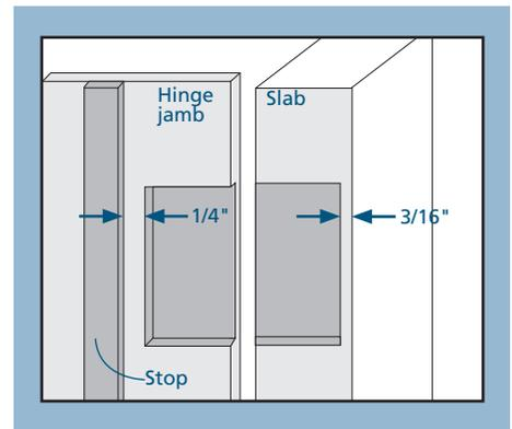
6. Using a template, mark the jambs and slab where the hinges will be mounted. Using a chisel or router, notch the jamb and slab for the outline of the hinge leaves and no deeper than the thickness of the leaves.
