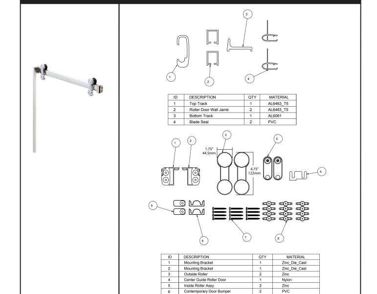
MATERIALS: Anodized Aluminum Excursions (Track) and Zinc Die Cast (Mounting Brackets). Bronze Finish is Powder Coated.
